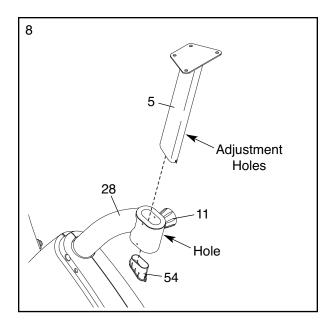
Attach the Seat (12) to the Seat Post (5) with four M8
